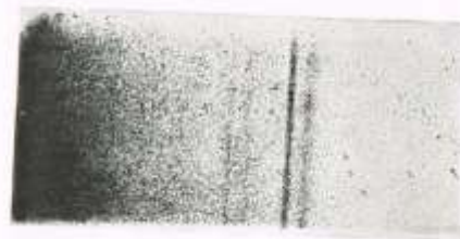
FIG. 30.—THE COMPTON EFFECT The photograph shows the change of wave-length of ether-waves, lines blue toward red, because of scattering by free electrons. \alpha and \beta are the initial characteristic X-ray lines of molybdenum, \alpha' and \beta' these same lines after suffering scattering in aluminum.
